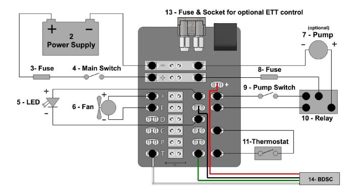
NOTE: When using the modular thermostat connection (#13) there are no connections on thermostat terminals (#11).
